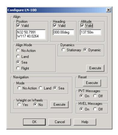
This dialog box is used primarily for sending configuration commands to the LN-100 unit. You can select the desired options and click the appropriate Execute button to send the configurations to the unit. You can also send PVT and/or HVEL messages to the unit at 1 second intervals by selecting the appropriate On radio button(s). For more information on the various configuration options refer to the LN-100 documentation.
